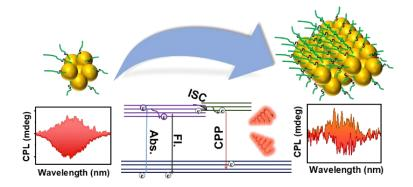
Scheme illustrating circularly polarised phosphorescence in monomeric and aggregated states of gold clusters.
