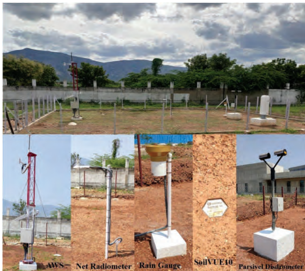
▲ Deep convective clouds before the occurrence of heavy rainfall event on 11 th November 2021 over Yerpedu, IISER Tirupati Permanent campus. Installed instruments, i.e., Automatic weather station, Rain Gauge, SoilVUE10, Net Radiometer, Parsivel Disdroemter are shown.
