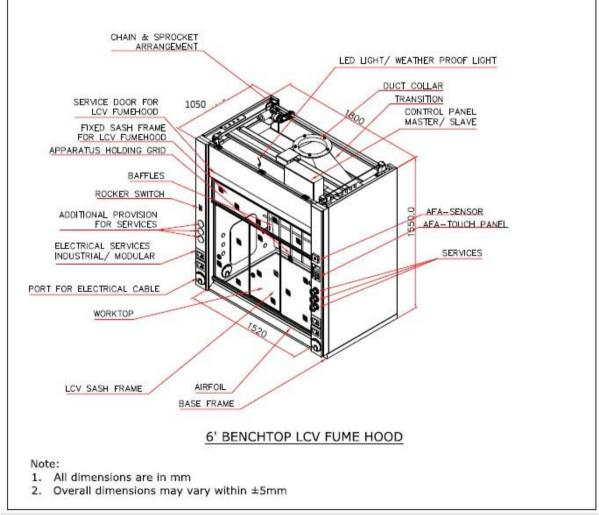
Superstructure Frame: It shall be a free-standing rigid panel structure of steel (G.I.)
